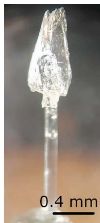
Figure 4 The single crystal of thiourea used for the TDS experiments, mounted on a glass fibre.
