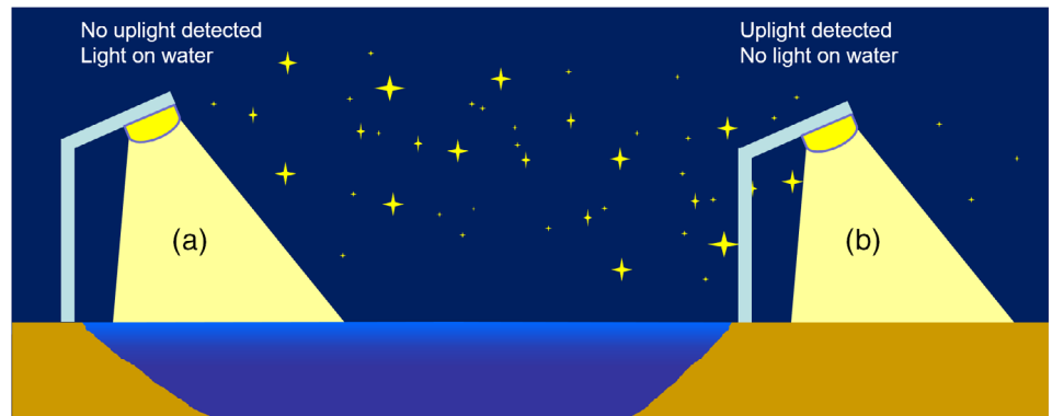
FIGURE 6 Two different shoreline lighting scenarios with the same luminaire
