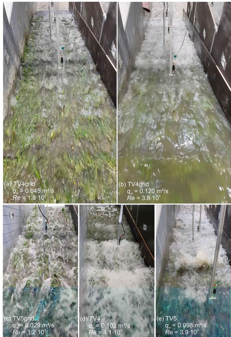
Figure 3. Photos of air-water flow patterns along the vegetated chutes. (a), (b), and (e) view in flow direction; (c) and (d) view against flow direction.
