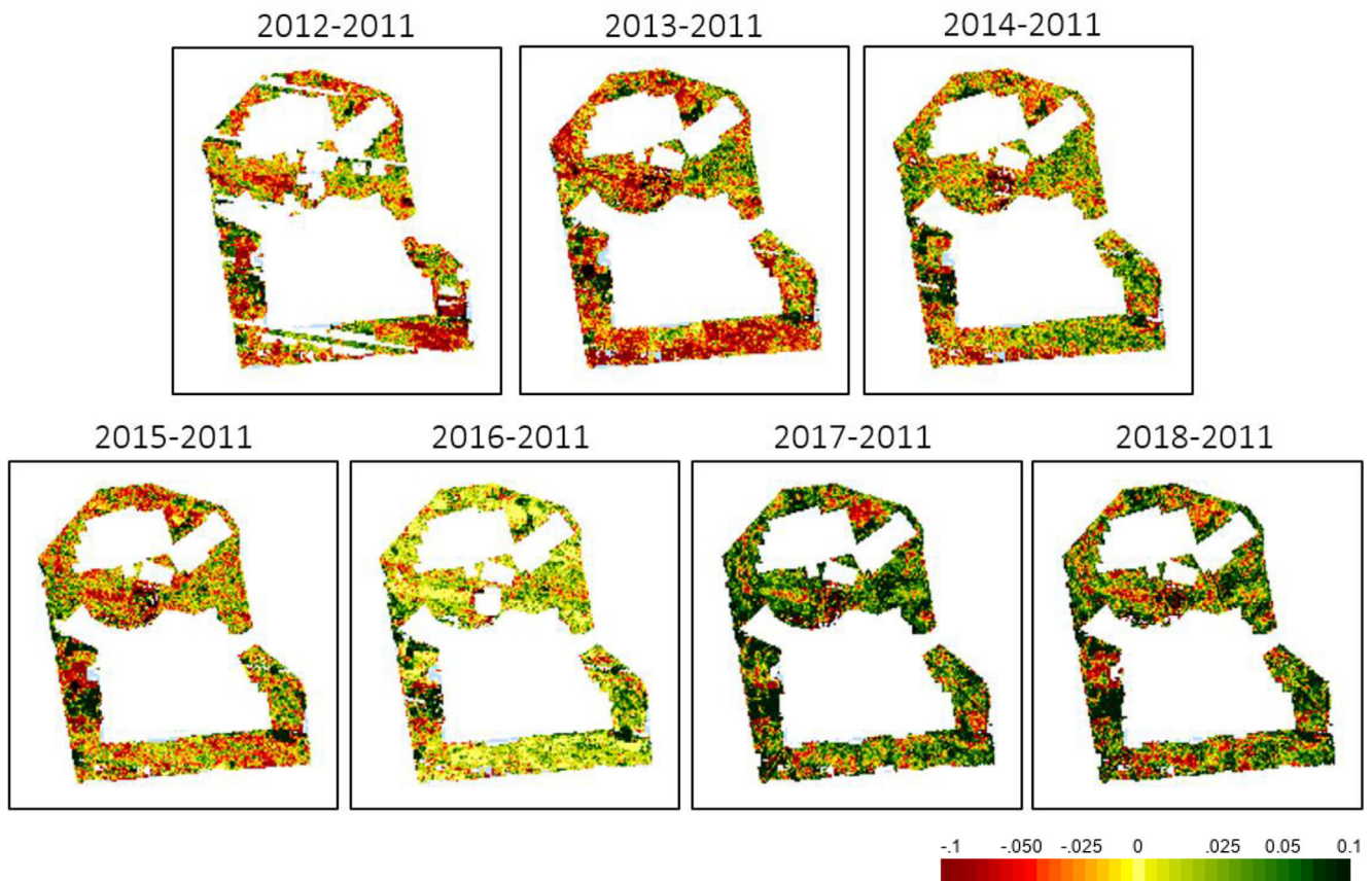
FIGURE 10 NDVI changes over the years compared to 2011. The first 5 years use Landsat 7 ETM+ data and the remaining 2 years use Landsat 8 OLI
