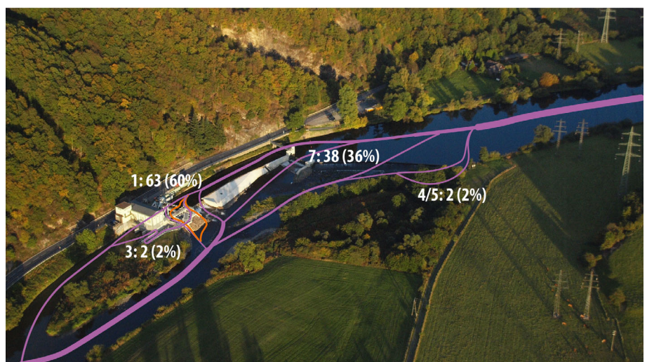
FIGURE 3 Number and proportion of smolts using the different migration routes past the power station. Route numbers refer to lower panel in Figure 2
