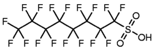
FIGURE 1: One of the common per- and polyfluoralkyl substances—perfluorooctane sulfonic acid (US Environmental Protection Agency 2019).
