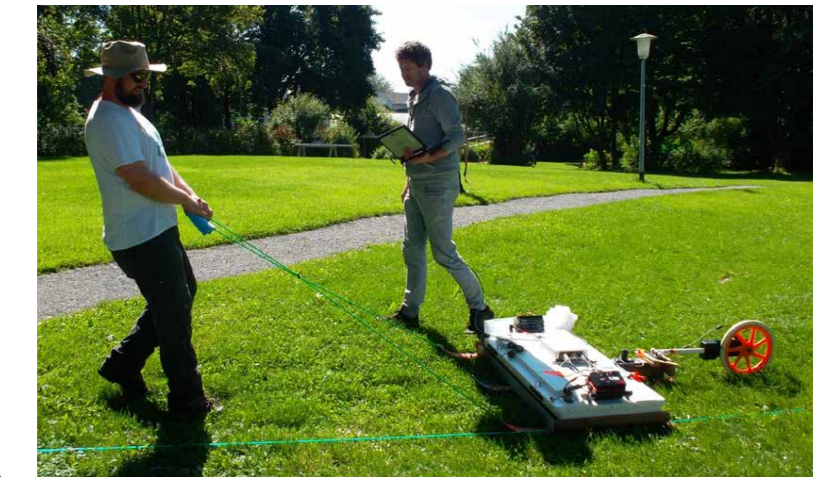
Fig. 4: The IDS Stream-C array mounted onto a self-built sled in action at the test site in Kempten.
