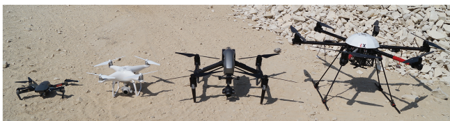
FIGURE 2 Tested UAS: Mavic Pro, Phantom 4 Pro+, Inspire 2 and XR6 (from left to right) [Color figure can be viewed at wileyonlinelibrary.com ]
