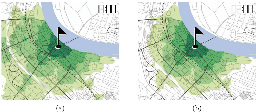
FIGURE 22 Continuation of the case study. (a) Travel times with start time Monday 6 p.m. (b) Travel times with start time Tuesday 2 a.m.
