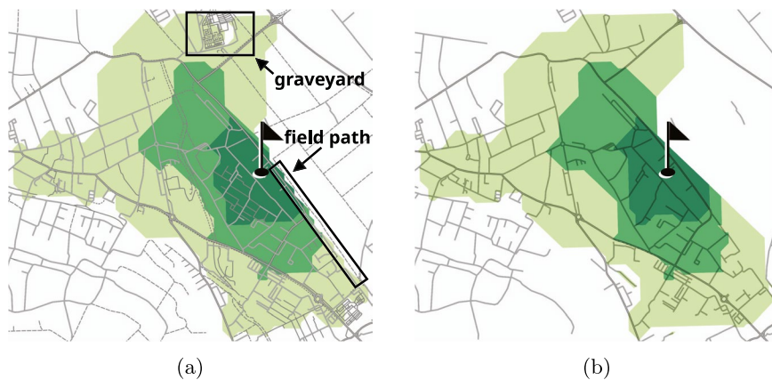
FIGURE 15 Generalization of time zones for different zoom levels. (a) Small streets yield an octilinear polygon with many bends. (b) Minor roads are ignored resulting in a SCHEMATIZATION with fewer bends
