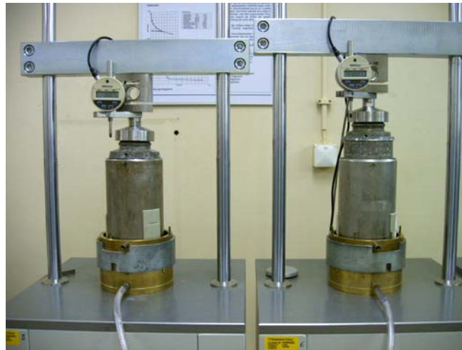
Fig. 3-1. Preconsolidation Tests of Kaolin
