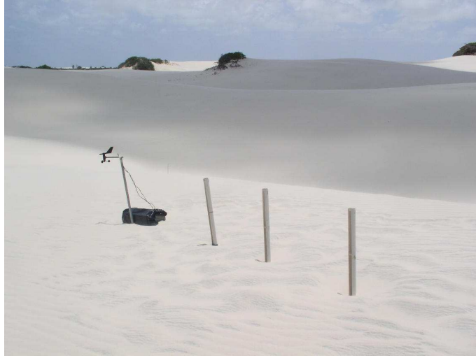
Figure 4.10: Measuring wind velocity and sand flux using an anemometer and the three traps at the different points of dune 3 in fig. 4.6.
