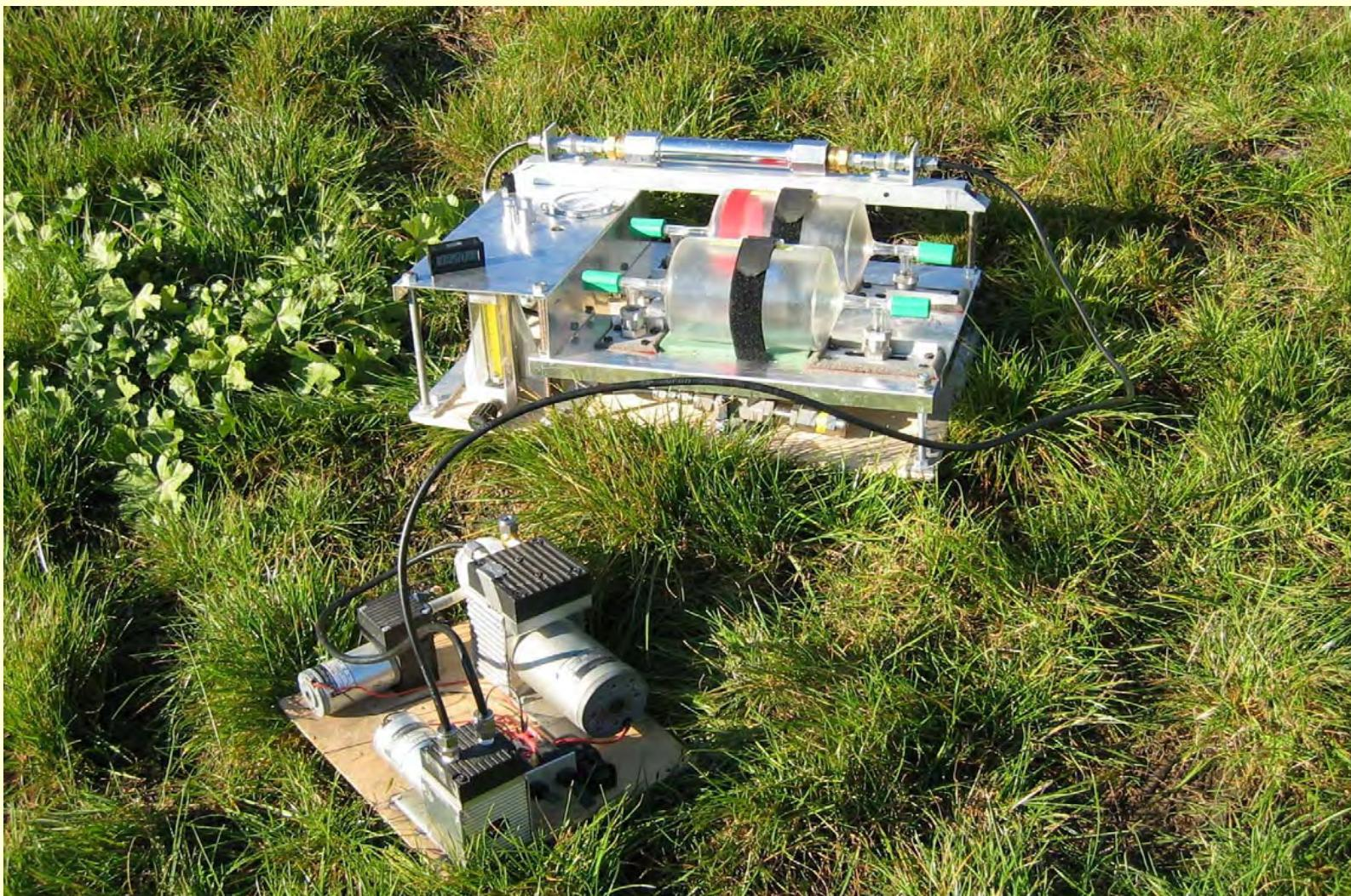
**Figure 1**    Flask Sampling System used for the ground reference sampling.
