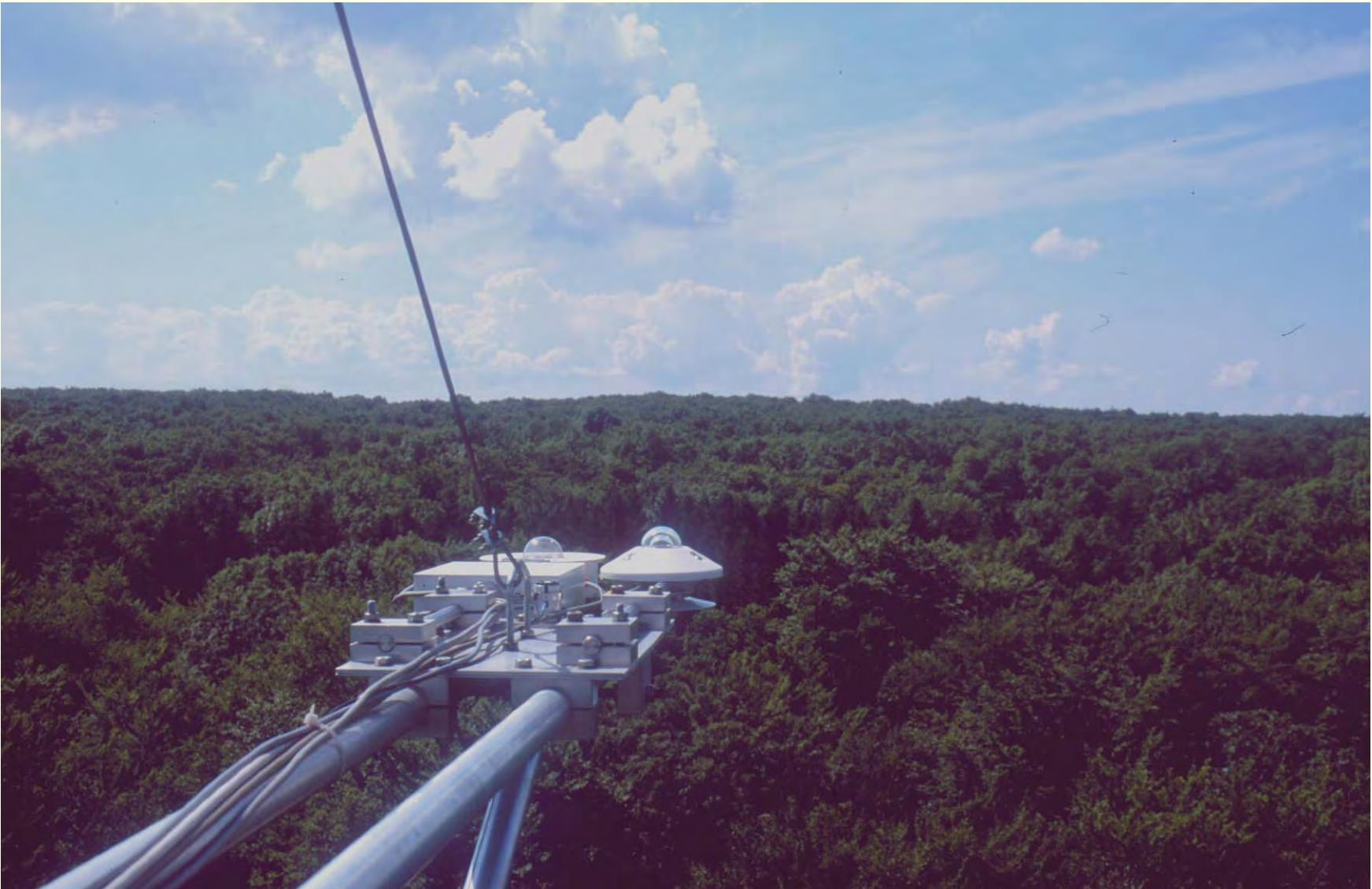
**Figure 4** View from the Hainich Tower over the canopy to the South. Placed on the boom are the sensors for radiation measurements.
