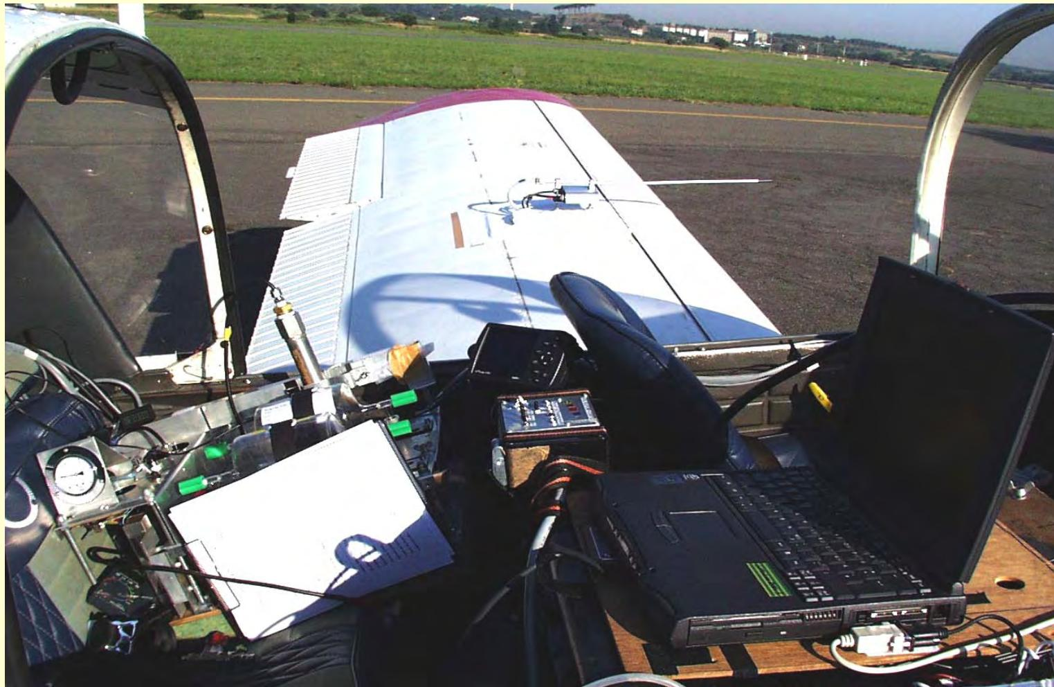
**Figure 7** FlightSamplingUnit, GPS (on the barrier between front and rear seat), switch box of the continuous measurement system in front of the GPS. Laptop for system controlling and data recording – during the flight fixed on the operators thigh. Sample flasks are stored in the rear of the cabin Recognizable are on the left wing the mounted sensors for air temperature and humidity, dynamic and static pressure and the compass module.
