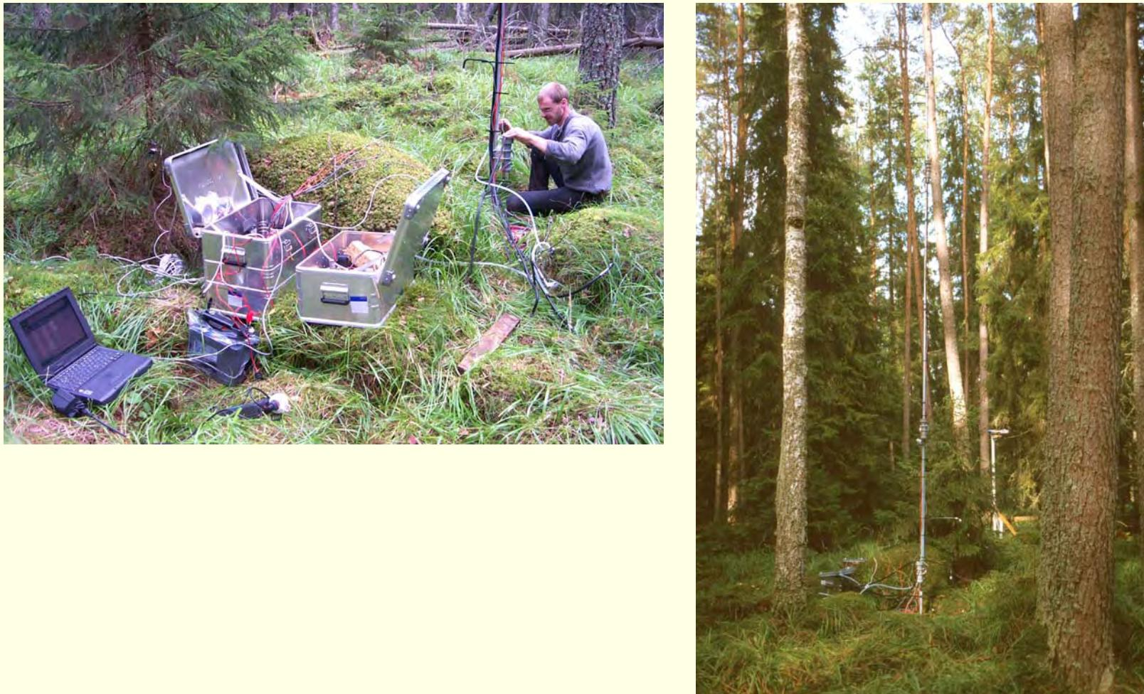
**Figure 6** Forest reference site. Installation of the sensors (left) and the operational measurement equipment.
