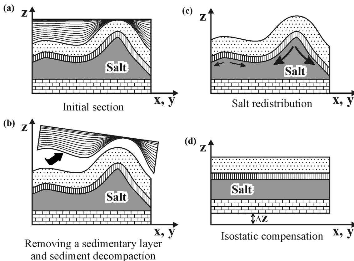
Figure 5.3. Schematic diagram showing steps of the reverse modelling from the initial state to the selected stratigraphic level (modified after Scheck et al., 2003).
