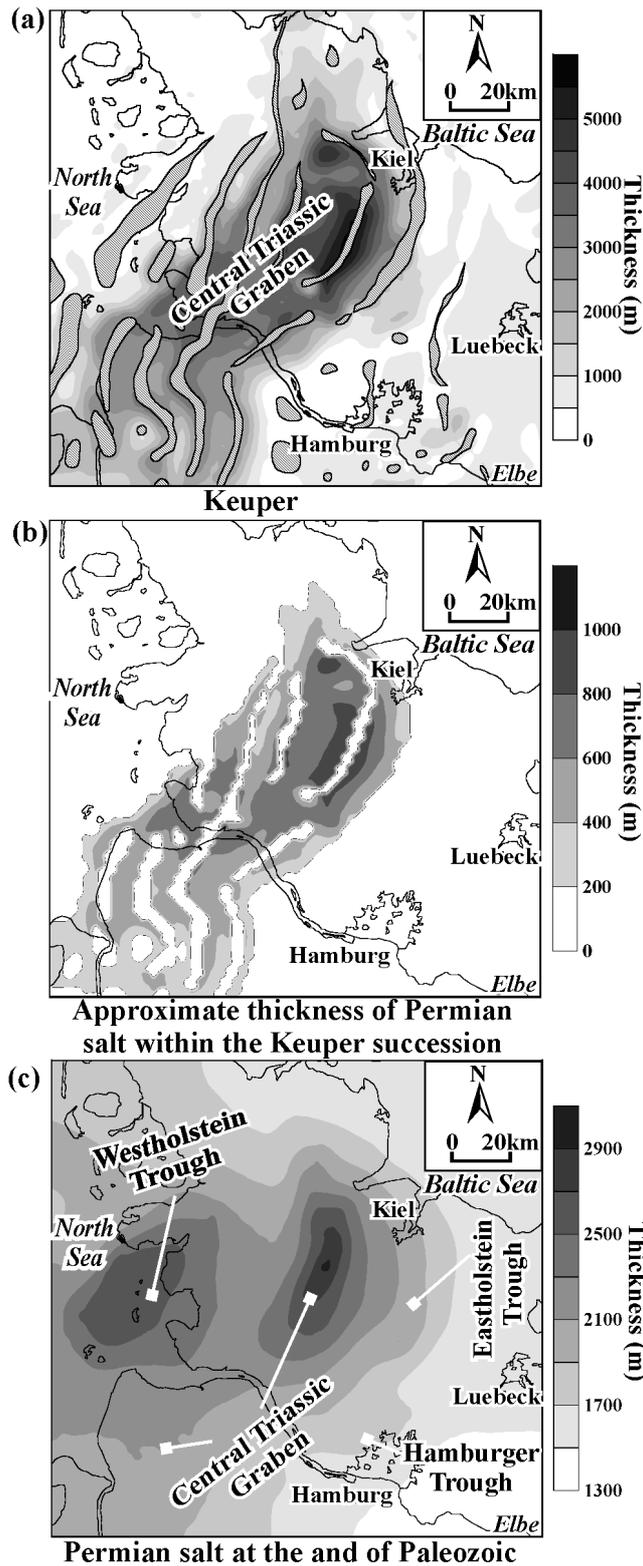
Figure 5.13. (a) Thickness map of the uppermost Middle Triassic and Upper Triassic (Keuper); (b) suggested thickness of the Permian salt within the Keuper strata; (d) reconstructed map of initial salt thickness obtained from 3D salt redistribution within the studied area.
