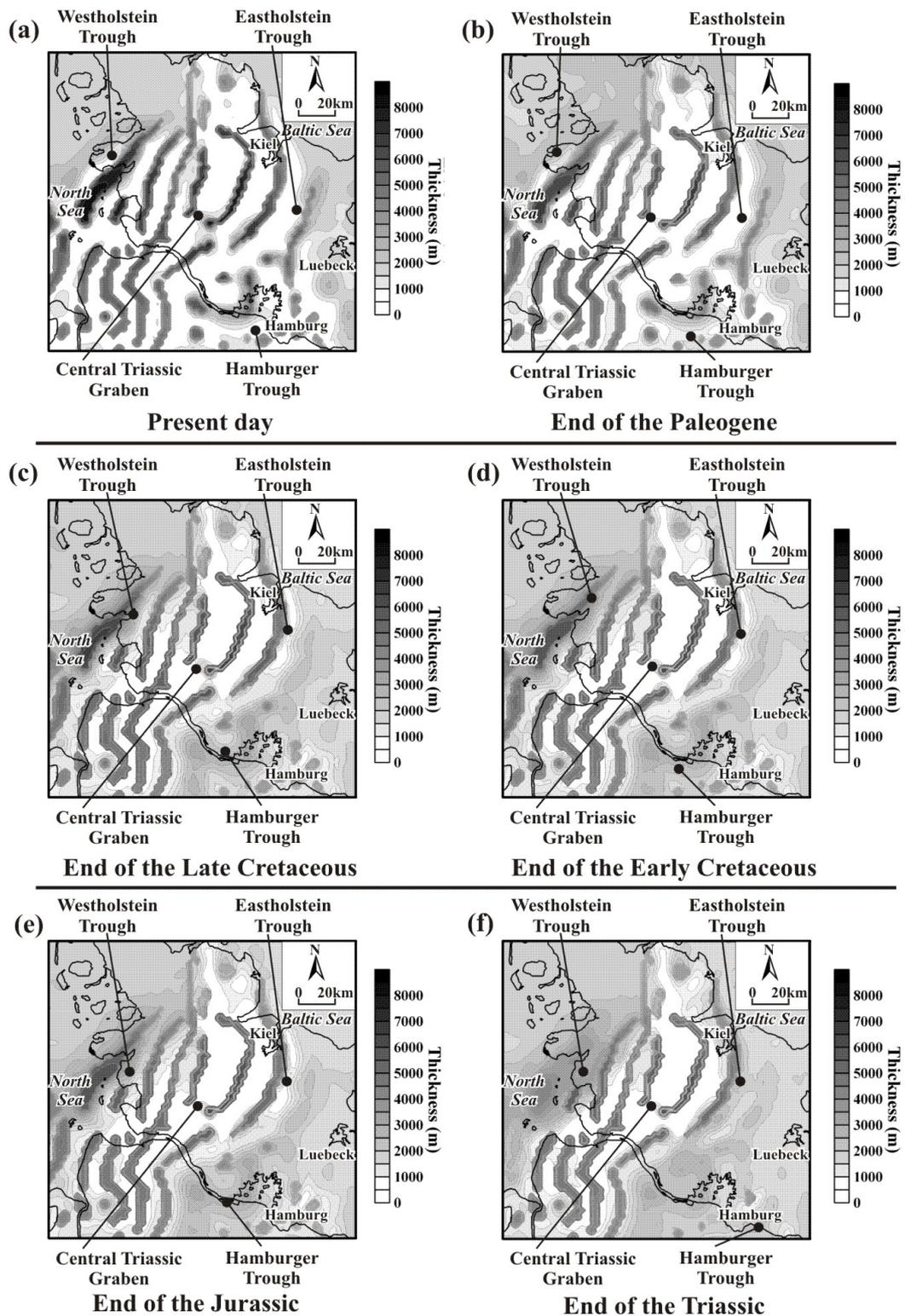
Figure 5.11. Isochore maps of the Permian salt representing thickness distribution of the salt from the end of the Triassic (f) to present-day (a) based on reverse modelling. Gradual movements of the depletion zone of Permian salt from the central part of the original Central Triassic Graben (f) towards its margins (a) is shown by white colour.
