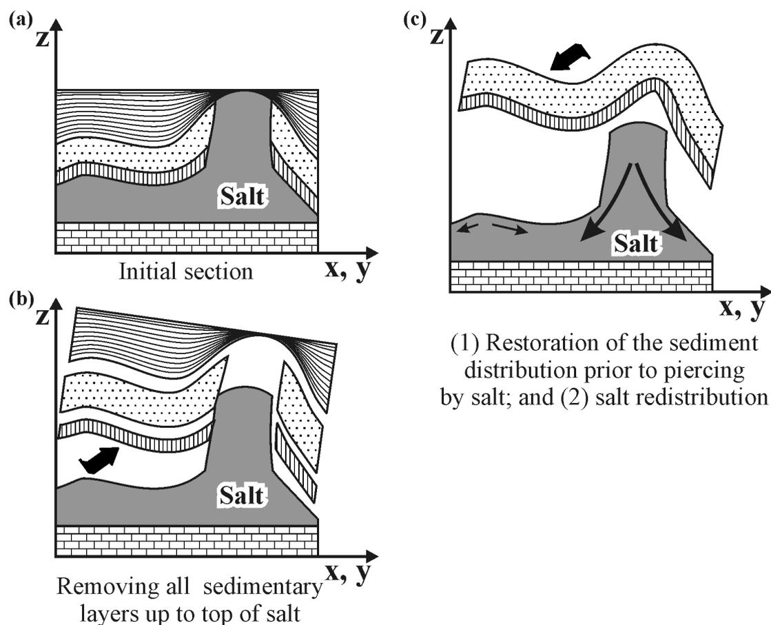
Figure 5.4. The schematic diagram shows a reconstruction of the sediment thickness prior to postdepositional erosion, allowing salt redistribution from the salt structure at the selected stratigraphic level (modified after Scheck et al., 2003).
