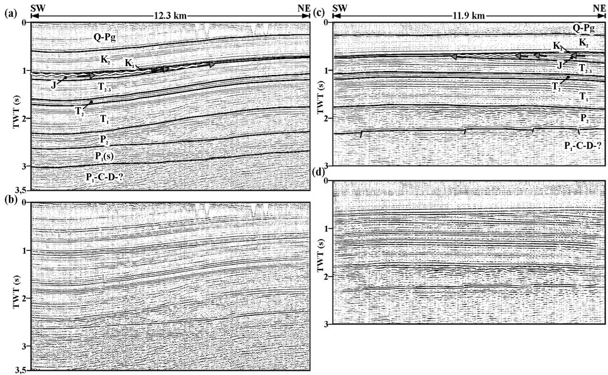
Figure 3.4. Interpreted seismic profiles 3 and 4. A typical structure from the NE part of the SE flank of the basin (Eastholstei-Mecklenburg block) is shown (visible erosional unconformity is indicated by wavy lines). See Fig. 3.1 for location. For stratigraphic key see Figure 3.2.
