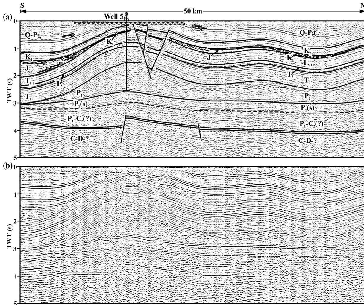
Figure 3.5. Interpretation of line 5 showing structural features along the Eastholstein-Mecklenburg block (visible erosional unconformities are indicated by wavy lines; arrows show on- and toplap of the reflection terminations). Late Carboniferous-Early Permian extension tectonics is shown beneath Permian salt pillow. See Fig. 3.1 for location. For stratigraphic key see Figure 3.2.
