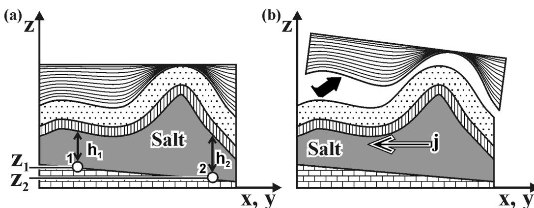
Figure 5.2. (a) Pressure balancing above the variable base topography of the salt layer. Calculation is performed by taking into account the pressure balancing for the interval between two points  $Z_1$  and  $Z_2$  as a reference depth. (b) Salt redistribution under new load conditions due to removing layer from top. Salt flow is characterized by the formal flux  $j$  which operates as a flow of salt towards areas of load deficit (modified after Scheck et al., 2003).
