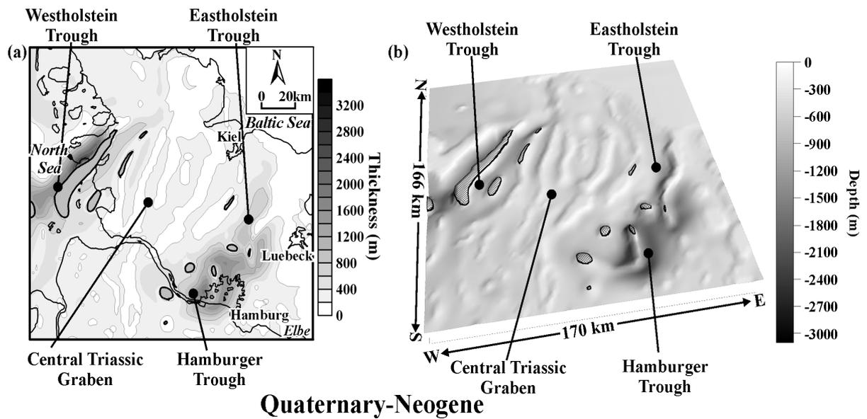
Figure 4.9. (a) Present-day thickness map of the Quaternary-Neogene. (b) Present-day depth position of the base of the Quaternary-Neogene, taken from the 3D structural model of the GG.
