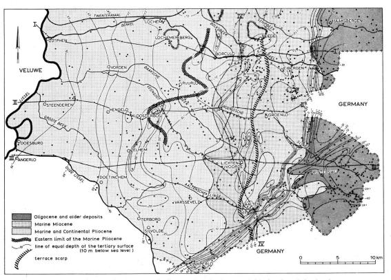
Fig. 4. Oligocene, Miocene and Pliocene deposits in East Gelderland, and the depth of their surface with respect to sea level.
