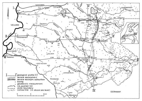
Fig. 1. Map of East Gelderland, showing the general topography, the location of the borings, geoelectrical measurements and geological sections.
