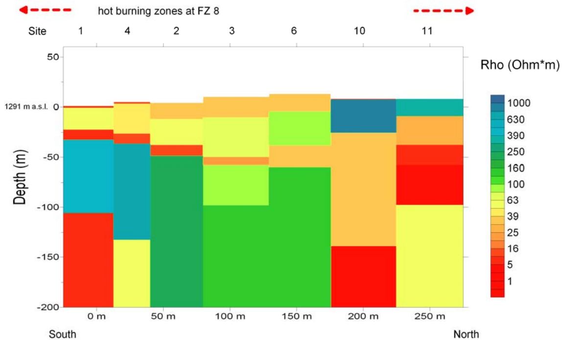
Figure 5: Resistivity-depth section from one-dimensional inversion of TEM data along profile no. 6 from south to north. The burning zone is marked by a dashed red line. The conductor is dipping northward from about 25 m down to 50 m depth.
