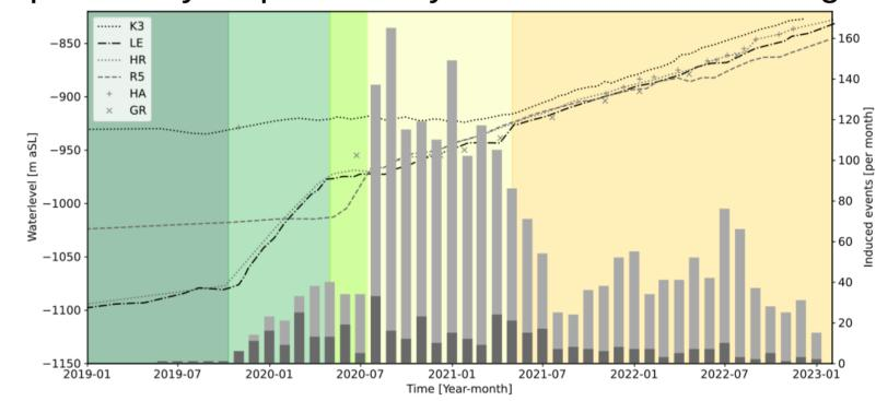
Phases of minewater rise combined with number of detected microseismic even
