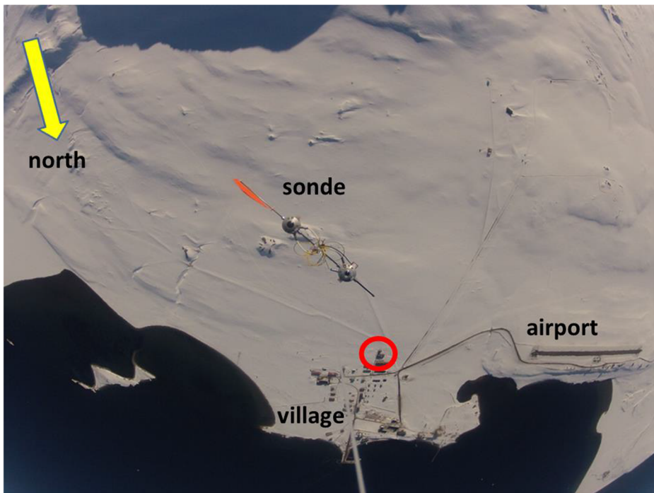
Fig. 2 Ny-Ålesund and the surroundings, seen from 1300 m aboveground on May 13, 2015. The sonde is fixed at the tether line 3 m below the camera. The center of the red circle marks the location of the balloon hall, associated to the observatory, being the starting point of the soundings
