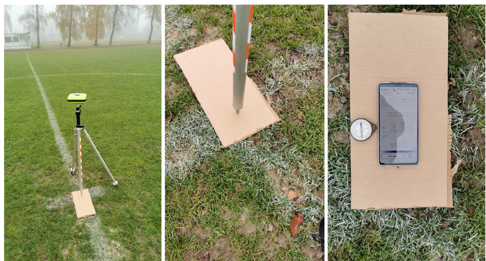
Fig. 8 Soccer field setup. Left and middle panel: the geodetic receiver has been used to compute the correct reference position of the smartphone. Right panel: the Mate20X has been aligned to geographic north, with the bottom edge eccentric over the reference point (the hole in the piece of cardboard)
