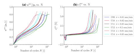
**Fig. 8** Undrained cyclic tests with different displacement rates (OCR<sub>0</sub> = 1,  $p_0$  = 200 kPa,  $\eta_0$  = 0,  $q_{ampl}$  = 45 kPa): a) normalized accumulated pore water pressure  $u^{acc}/p_0$  as a function of the number of cycles and b) accumulated axial strain as a function of the number of cycles (simulation=solid lines, experiment=dashed lines)
