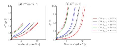
Fig. 14 Undrained cyclic tests with different deviatoric amplitudes on samples consolidated anisotropically (OCR<sub>0</sub> = 1,  $p_0$  = 200 kPa,  $\eta_0$  = 0.375): **a** normalized accumulated pore water pressure  $u^{\text{acc}}/p_0$  as a function of the number of cycles and **b** accumulated axial strain as a function of the number of cycles (simulation = solid lines, experiment = dashed lines)
