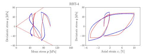
Fig. 17 Effective stress path and deviatoric stress—axial strain relations for the undrained cyclic test RBT-4 on Lower Rhine Clay with  $q_{ampl} = 60$  kPa and  $\dot{s} = 0.02$  mm/min (simulation = red, experiment = blue) (color figure online)
