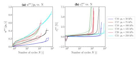
Fig. 10 Undrained cyclic tests with variation of the initial mean pressure (OCR<sub>0</sub> = 1,  $\eta_0$  = 0,  $\dot{s}$  = 0.1 mm/min): **a** normalized accumulated pore water pressure  $u^{acc}/p_0$  as a function of the number of cycles and **b** accumulated axial strain as a function of the number of cycles (simulation = solid lines, experiment = dashed lines)
