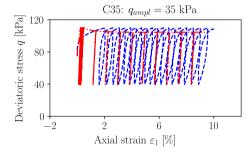
**Fig. 13** Deviatoric stress vs. axial strain in undrained cyclic tests with different deviatoric amplitudes on samples consolidated anisotropically (OCR<sub>0</sub> = 1,  $p_0$  = 200 kPa,  $\eta_0$  = 0.375) (simulation = red, experiment = blue) (color figure online)
