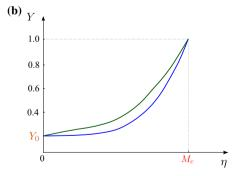
**Fig. 2** Definition of the degree of nonlinearity: **a** contour plot of Y in p-q space, **b** Y in dependence on the stress ratio  $\eta$  (green = Y from the reference model [9], blue = Y proposed in Eq. (24)) (color figure online)
