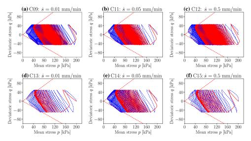
Fig. 6 Effective stress paths in undrained cyclic tests with different displacement rates (OCR<sub>0</sub> = 1,  $p_0$  = 200 kPa,  $\eta_0$  = 0,  $q_{ampl}$  = 45 kPa) (simulation = red, experiment = blue) (color figure online)
