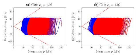
Fig. 15 Effective stress paths in undrained cyclic tests with samples cut out in horizontal direction (OCR<sub>0</sub>  $\approx$  1,  $p_0 = 100$ , kPa,  $\eta_0 = 0$ ,  $q_{ampl} = 45$  kPa,  $\dot{s} = 0.1$  mm/min) (simulation = red, experiment = blue) (color figure online)
