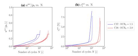
Fig. 11 Undrained cyclic tests with variation of the initial overconsolidation ratio ( $p_0 = 100$ , kPa,  $q_{ampl} = 30$  kPa,  $\eta_0 = 0$ ,  $\dot{s} = 0.1$  mm/min): a normalized accumulated pore water pressure  $u^{acc}/p_0$  as a function of the number of cycles and **b** accumulated axial strain as a function of the number of cycles (simulation = solid lines, experiment = dashed lines)
