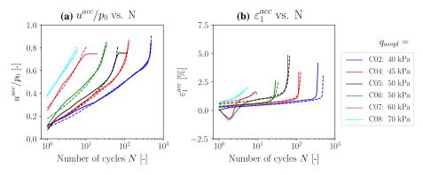
Fig. 5 Undrained cyclic tests with different stress amplitudes (OCR<sub>0</sub> = 1,  $p_0$  = 200 kPa,  $\eta_0$  = 0,  $\dot{s}$  = 0.1 mm/min): a normalized accumulated pore water pressure  $u^{\rm acc}/p_0$  as a function of the number of cycles and **b** accumulated axial strain as a function of the number of cycles (simulation = solid lines, experiment = dashed lines)
