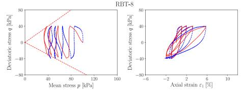
Fig. 20 Effective stress path and deviatoric stress-axial strain relations for the undrained cyclic test RBT-8 on Lower Rhine Clay with  $q_{ampl} = 40$  kPa and  $\dot{s} = 0.02$  mm/min (simulation = red, experiment = blue) (color figure online)
