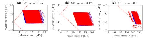
Fig. 12 Effective stress paths in undrained cyclic tests with variation of the initial stress ratio (OCR<sub>0</sub> = 1,  $p_0$  = 200, kPa  $\dot{s}$  = 0.1 mm/min) (simulation = red, experiment = blue) (color figure online)
