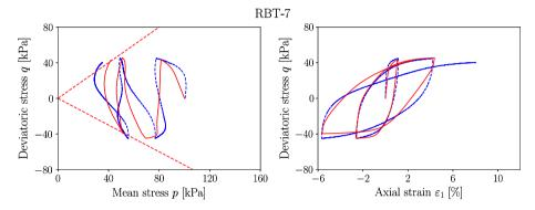
Fig. 19 Effective stress path and deviatoric stress-axial strain relations for the undrained cyclic test RBT-7 on Lower Rhine Clay with  $q_{ampl} = 45$  kPa and  $\dot{s} = 0.02$  mm/min (simulation = red, experiment = blue) (color figure online)
