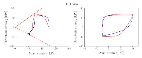
Fig. 18 Effective stress path and deviatoric stress-axial strain relations for the undrained cyclic test RBT-5w on Lower Rhine Clay with  $q_{\text{ampl}} = 60 \text{ kPa}$  and  $\dot{s} = 0.05 \text{ mm/min}$  (simulation = red, experiment = blue) (color figure online)
