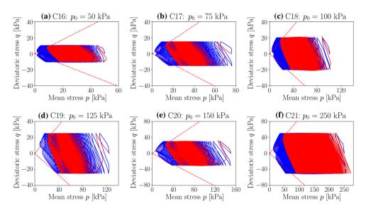
Fig. 9 Effective stress paths in undrained cyclic tests with variation of the initial mean pressure (OCR<sub>0</sub> = 1,  $\eta_0$  = 0,  $\dot{s}$  = 0.1 mm/min) (simulation = red, experiment = blue) (color figure online)
