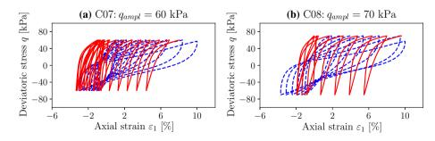
Fig. 4 Deviatoric stress vs. axial strain in undrained cyclic tests with different stress amplitudes (OCR<sub>0</sub> = 1,  $p_0$  = 200 kPa,  $\eta_0$  = 0,  $\dot{s}$  = 0.1 mm/min) (simulation = red, experiment = blue) (color figure online)
