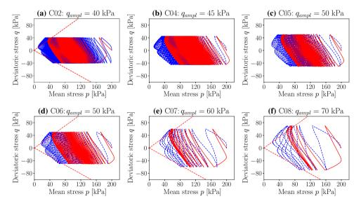
Fig. 3 Effective stress paths in undrained cyclic tests with different stress amplitudes (OCR<sub>0</sub> = 1,  $p_0$  = 200 kPa,  $\eta_0$  = 0,  $\dot{s}$  = 0.1 mm/min) (simulation = red, experiment = blue) (color figure online)
