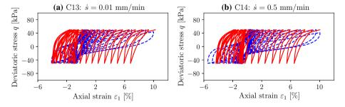
Fig. 7 Deviatoric stress versus axial strain in undrained cyclic tests with different displacement rates (OCR<sub>0</sub> = 1,  $p_0$  = 200 kPa,  $\eta_0$  = 0,  $q_{ampl}$  = 45 kPa) (simulation = red, experiment = blue) (color figure online)
