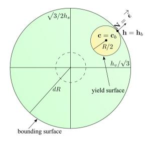
**Fig. 1** Yield surface and bounding surface of the extended ISA plasticity for clays (d = 2 has been used). Example when the intergranular strain is fully mobilized  $\mathbf{h} = \mathbf{h}_b$  and  $\mathbf{c} = \mathbf{c}_b$
