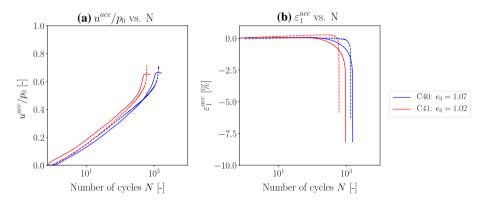
Fig. 16 Undrained cyclic tests with different deviatoric amplitudes samples cut out in horizontal direction (OCR<sub>0</sub>  $\approx 1$ ,  $p_0 = 100$ , kPa,  $\eta_0 = 0$ ,  $q_{\text{ampl}} = 45$  kPa,  $\dot{s} = 0.1$  mm/min): **a** normalized accumulated pore water pressure  $u^{\text{acc}}/p_0$  as a function of the number of cycles and **b** accumulated axial strain as a function of the number of cycles (simulation = solid lines, experiment = dashed lines)
