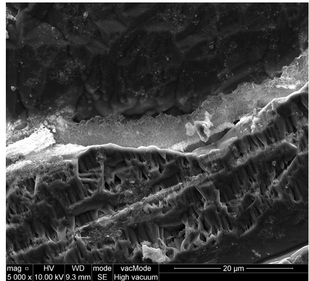
Fig. 17 SEM image clearly shows new calcium phosphates filling a microcrack among the calcite grains as a result of the DAP treatment
