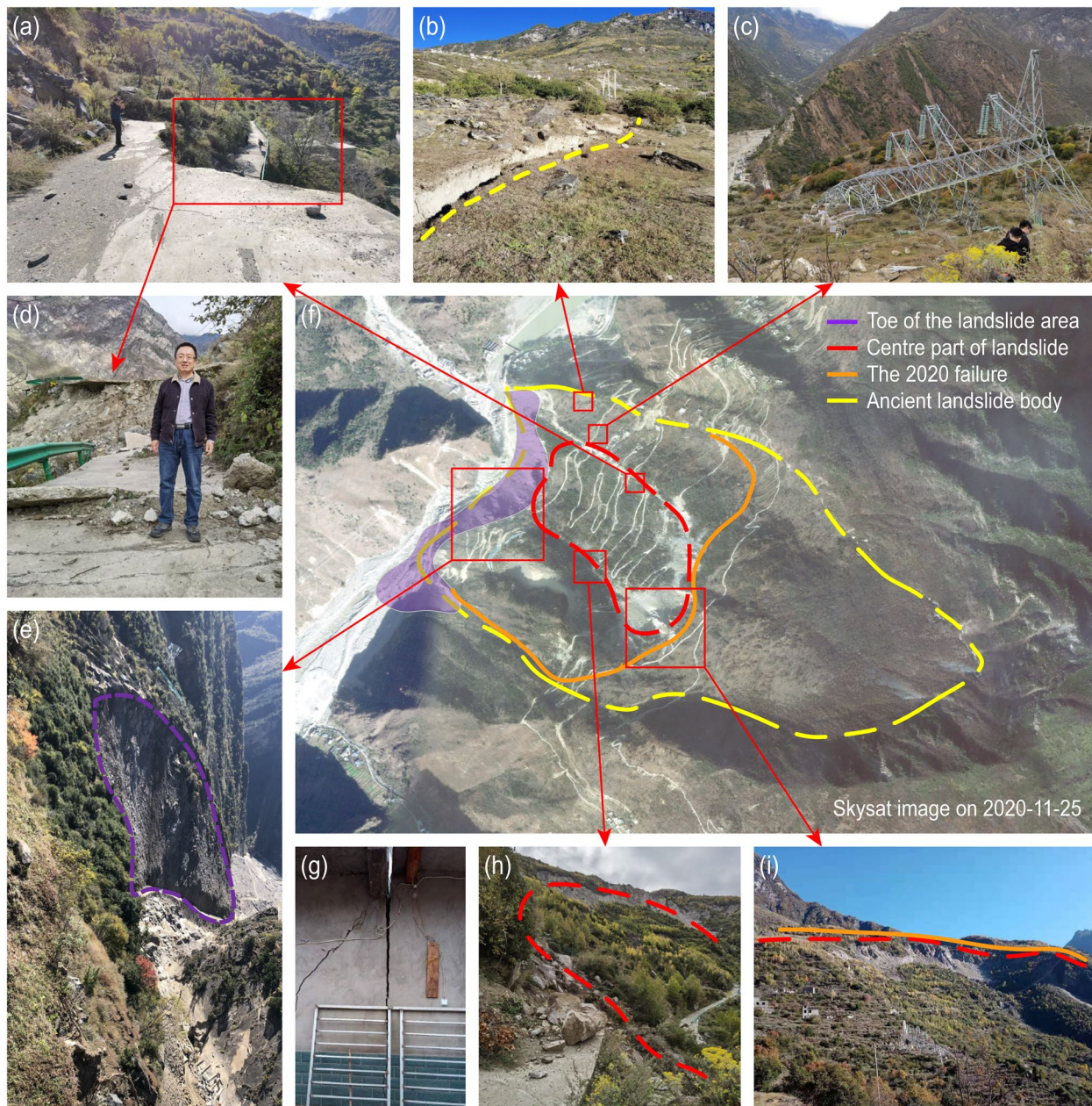
Fig. 2 Display of the landslide failure and different zones of the landslide body, as well as examples of damages in the event. (a) Ravaged roads on the edge of the central failure. (b) The northern lateral flank of the landslide. (c) Damaged EHV (Extra High Voltage) transmission tower. (d) Front view of ravaged roads. (e) The toe of the landslide body. (f) Skysat optical image acquired on 25 November 2020, with
