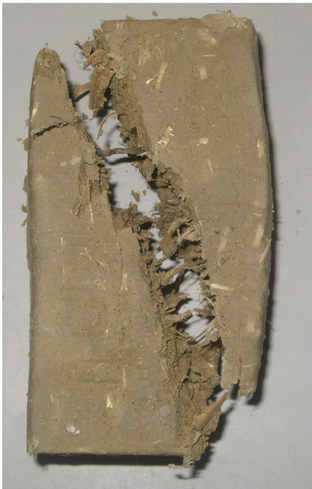
Fig. 13 Roughness of failure plane caused by straw filaments, fiber content = 1%
