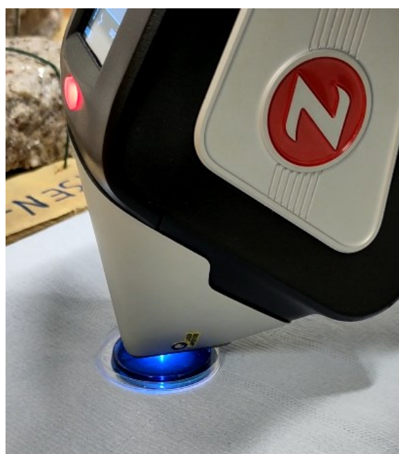
Fig. 1: pLIBS measurement on a fused bead containing Cu as dying agent.
