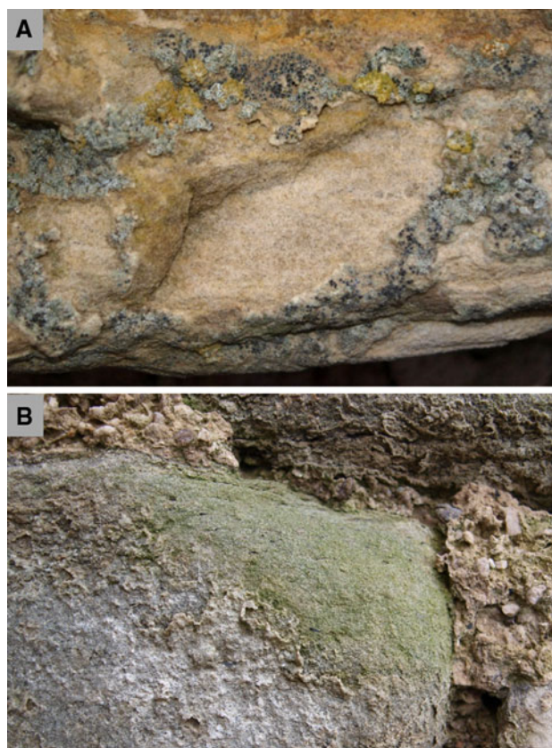
Fig. 3 Macroscopic appearance of (microbially) colonized sandstone surfaces. a Endolithic lichens in conjunction with scaling and backweathering of the surface. b Layer of green algae
