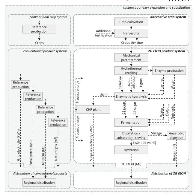
FIGURE 3 System boundaries and simplified flow diagram
