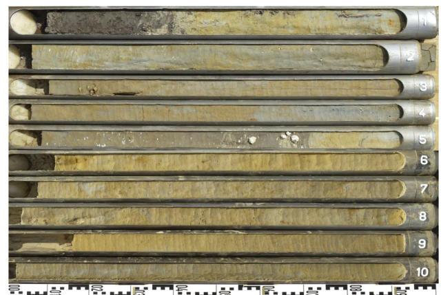
Figure 3. Photo of vibracore VRT 1. Upper left corner = ground surface; lower right corner = final drilling depth (10 m b.s.). The core is dominated by silty sediments with various amounts of clay. Note the distinct shift from clay-rich dark greyish silts towards light-brown greyish silts with decreasing clay contents at 4.71 m. Photo P. Fischer (27.04.2015). [Color figure can be viewed at wileyonlinelibrary.com ].
