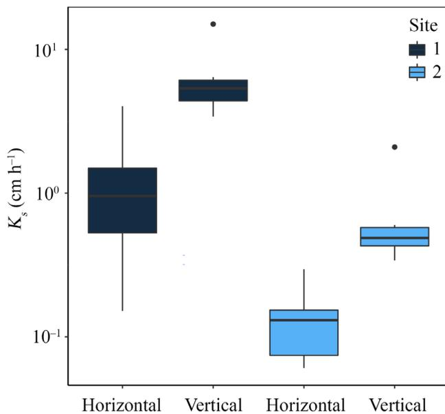
**FIGURE 2** Boxplot of saturated hydraulic conductivity ( $K_s$ , cm h<sup>-1</sup>) of peat soils in horizontal and vertical directions at site 1 and site 2
