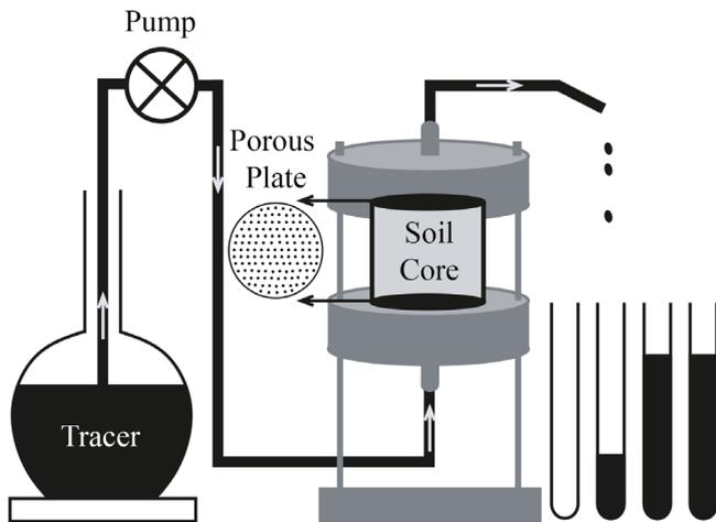
**FIGURE 1** Set-up for miscible displacement experiments in intact peat soil samples
