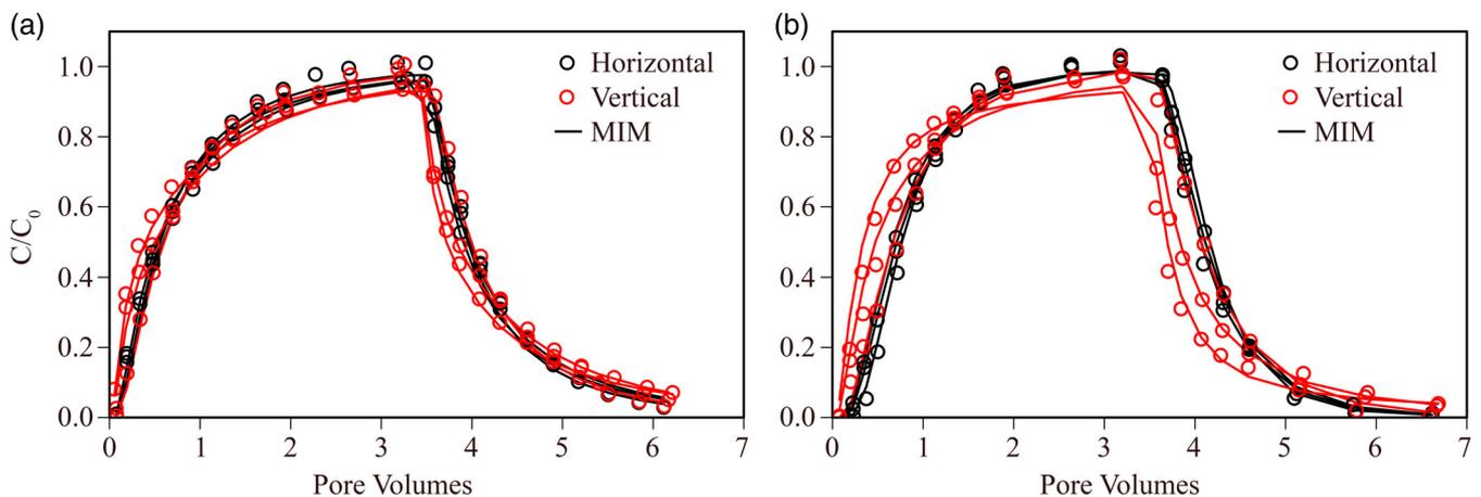
**FIGURE 3** Corrected bromide breakthrough curves plotted as relative concentrations ( $C/C_0$ ) against number of pore volumes: (a) site 1, (b) site 2. The solid lines show the mobile and immobile model (MIM)
