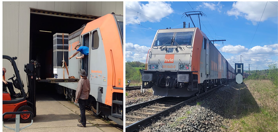
Figure 3. Assembling of the Rail-CRNS sensor into the BR 185 locomotive; here lifting the main unit (left) and the BR 185 while passing the meadow area (right).
