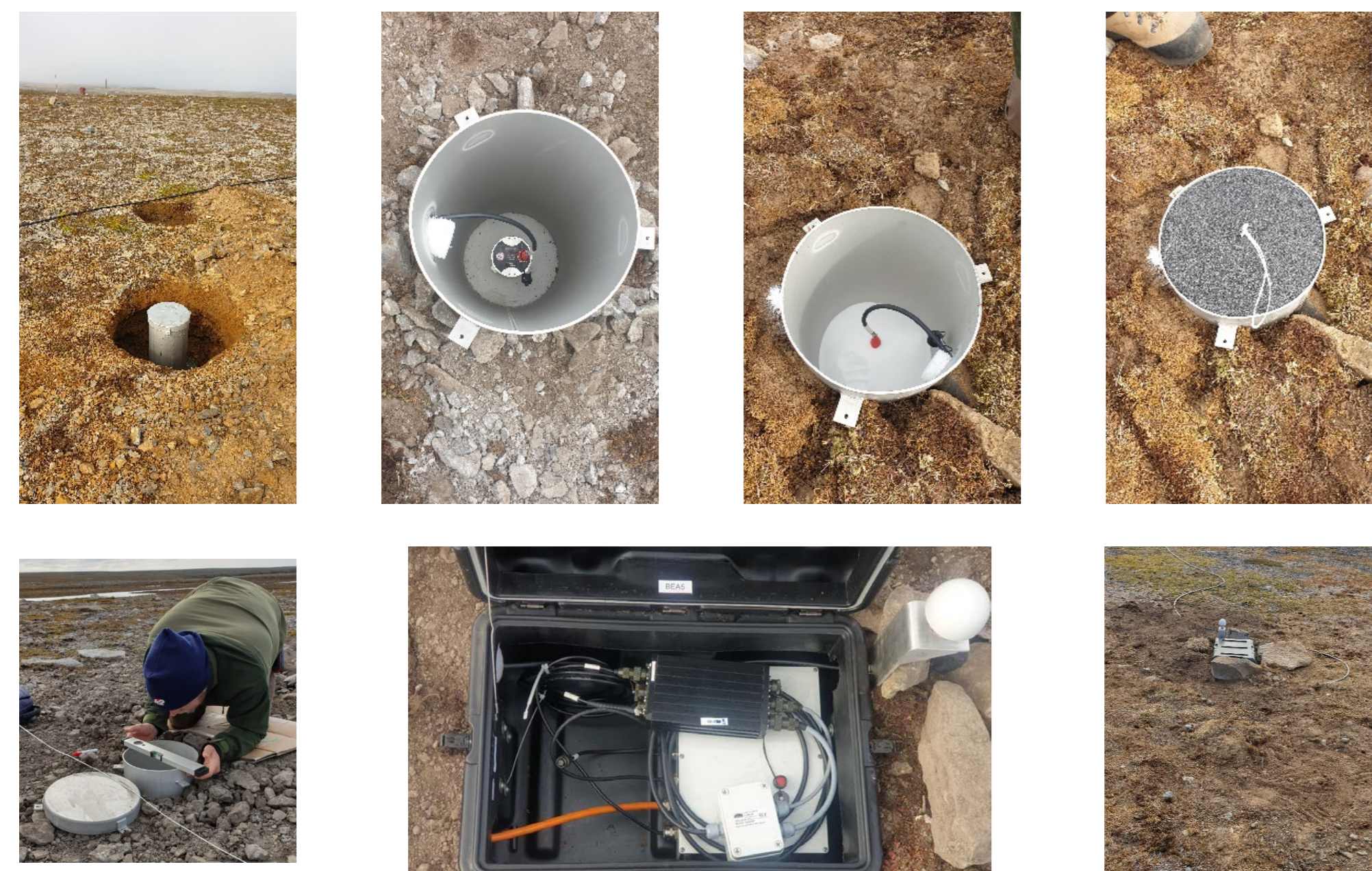
The seismometers were installed in a stainless-steel cylinder, oriented and covered with fine sand, the digitizers and modems were installed in a plastic box buried in the ground.
